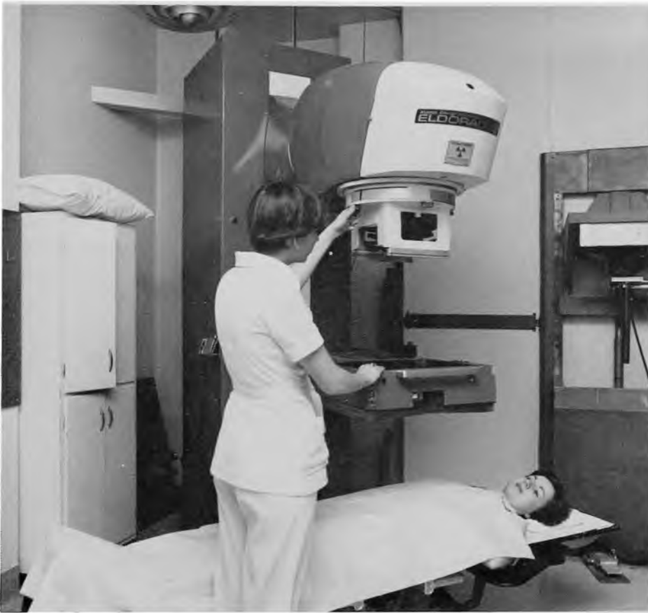
Figure 4-13. AECL pedestal cobalt 60 unit installed at the Ontario Cancer Institute and used almost exclusively for the irradiation of large complex shaped fields. The device for obtaining complex shaped fields is illustrated.
