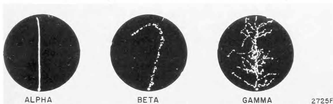
Figure 3-5. Cloud chamber photograph of alpha, beta, and gamma ray tracks. (J.B. Hoag: Electron and Nuclear Physics , courtesy D. Van Nostrand Co.) (H4)
