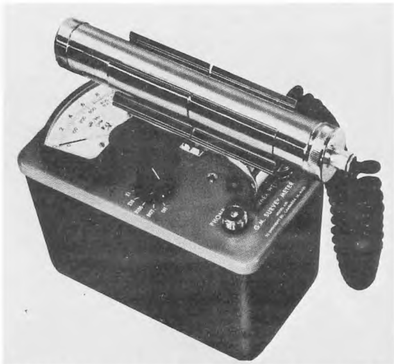
Fig 11-12. —Portable survey meter equipped with an end-window G-M tube. (Courtesy of Baird-Atomic, Inc.)
