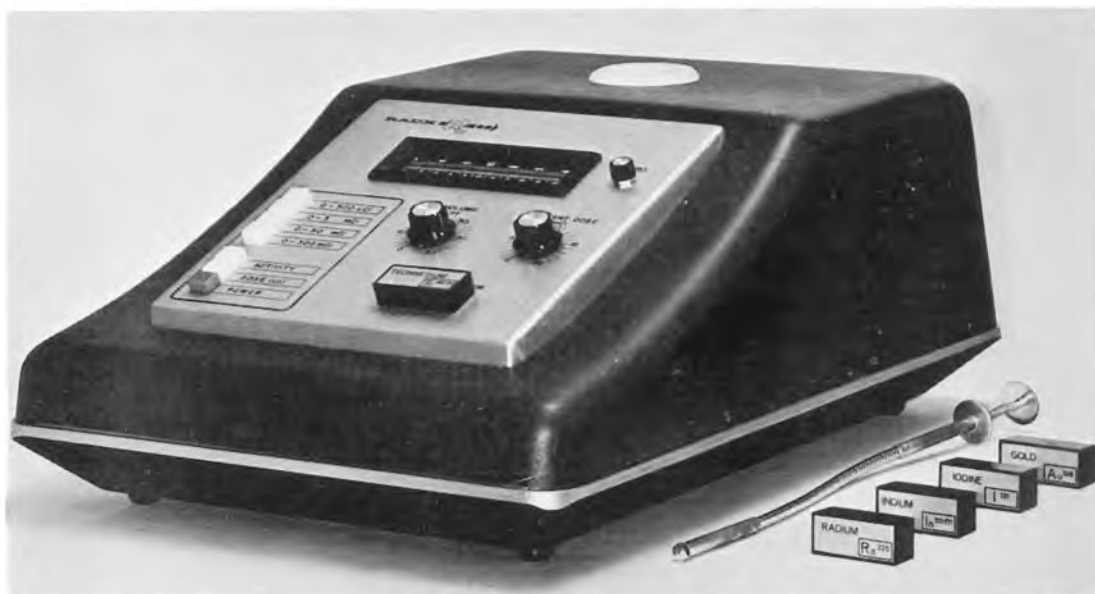
Fig 11-4. —Well-type ionization chamber and electrometer (isotope calibrator) used to measure the activity of a radioactive sample prior to administration of the sample to a patient. The volume of the sample to be administered is computed from the measured activity, often automatically by the isotope calibrator. (Courtesy of RADX Corp.)
