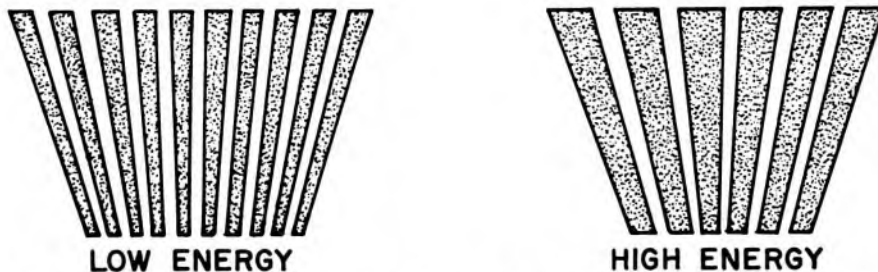
Fig 14-7. — Multihole focused collimators. Thicker lead septa are required to attenuate high-energy photons.
