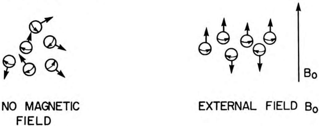
Figure 22.2 Alignment of nuclear spins in a magnetic field B_0 .
