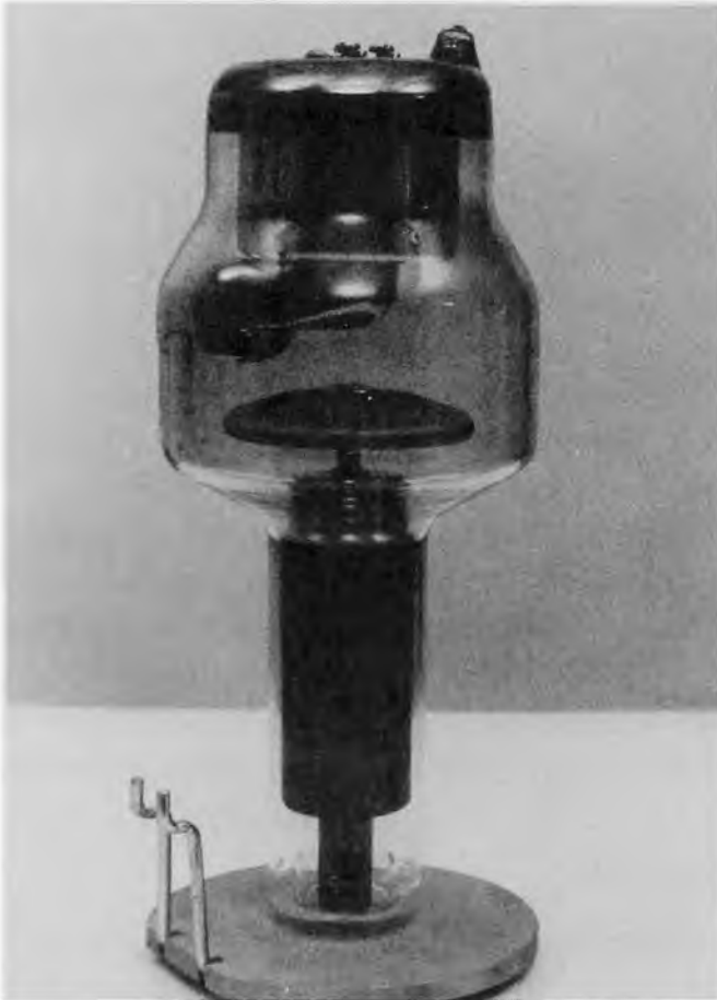
Figure 6.1. Rotating anode x-ray tube.
