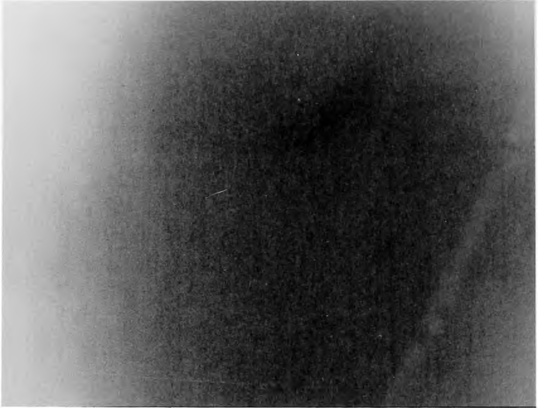
Figure 13.6. Grid cut-off due to upside down focused grid.
