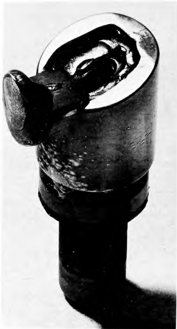
FIG. IV-7. Damage caused to x-ray tube anodes by excessively high electron flux.
