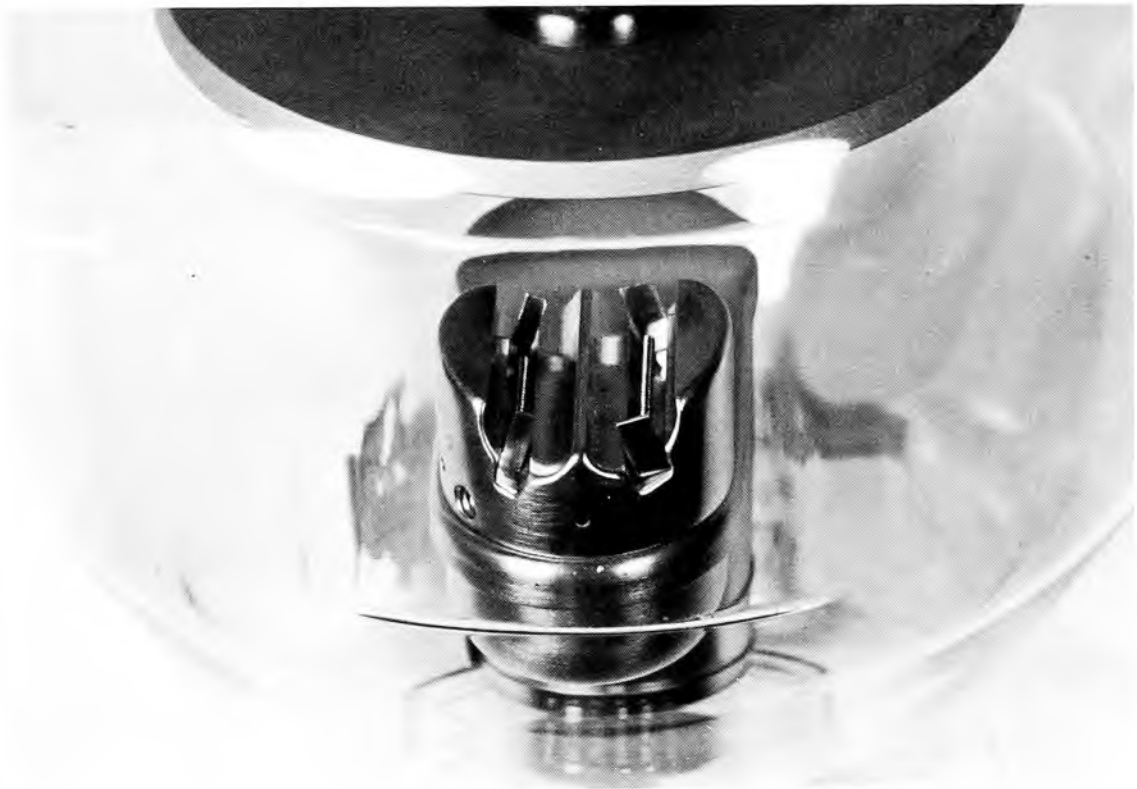
FIG. IV-6. Cathode structure of a modern double-focus rotating-anode x-ray tube. Each filament supplies electrons to a focus of different size. Note the focusing structure of the cathode.
