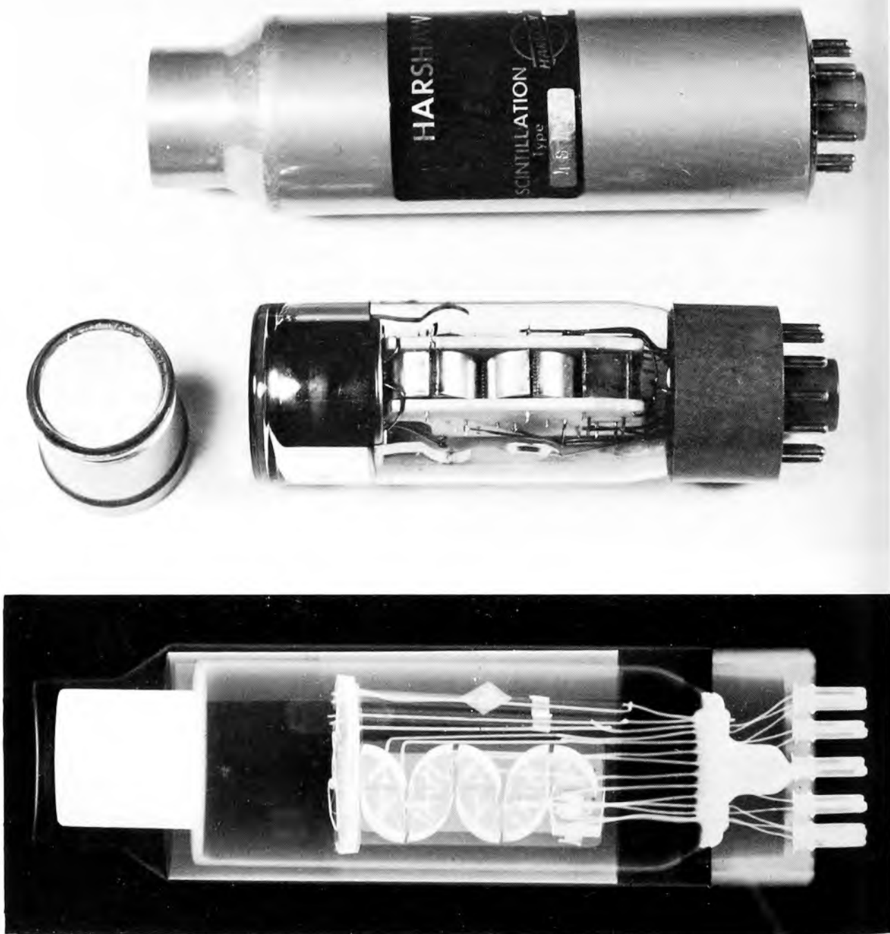
FIG. XI-9. Scintillation detector and component parts.
