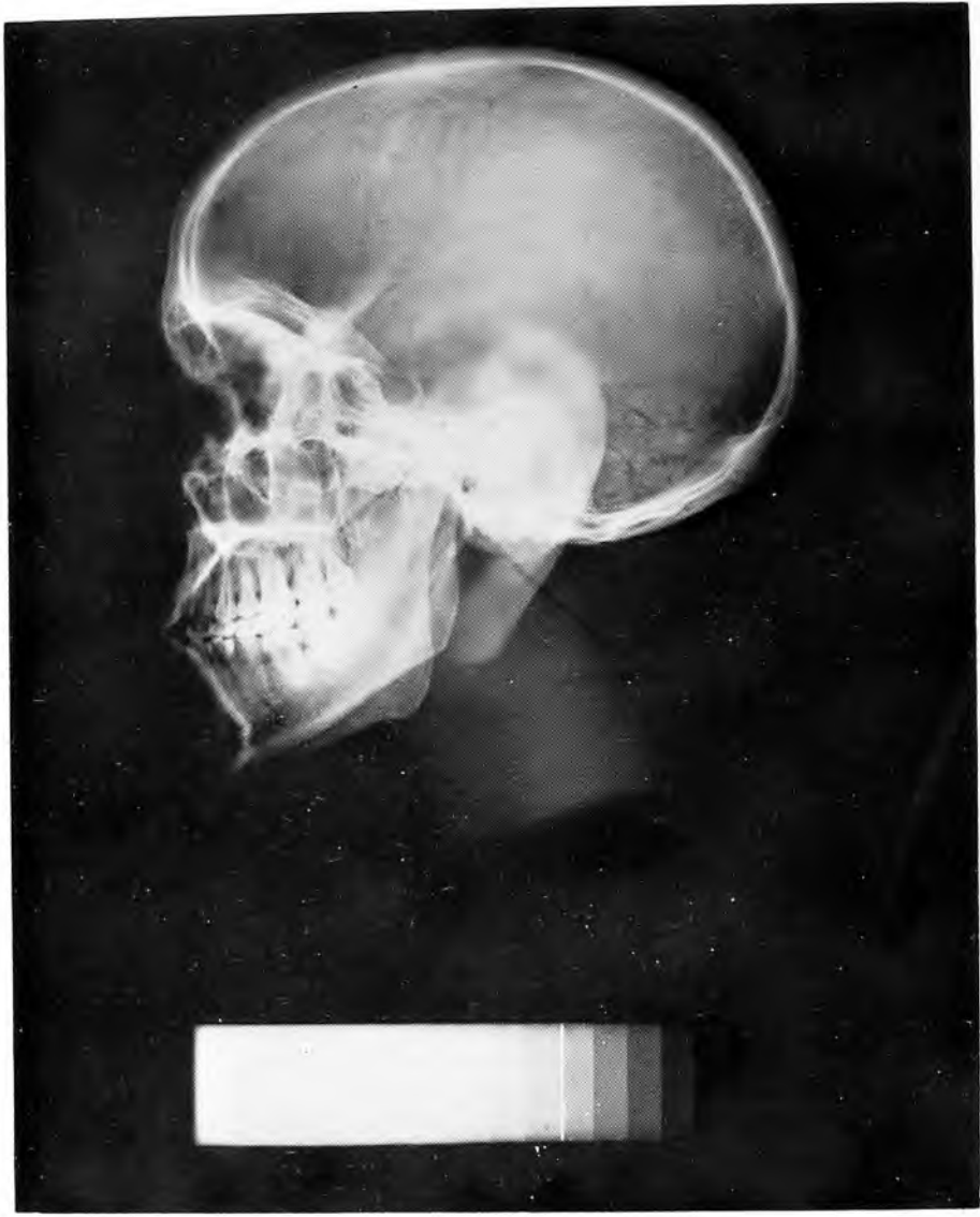
FIG. VI-18. Radiographs of the phantom of a head on films having different characteristic curves.
