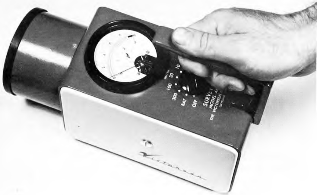
FIG. XI-6. Portable ionization chamber survey meter (Victoreen Survey Meter Model 440). Instrument is designed to measure exposure rates, and is mostly used for measuring stray x-radiation.
