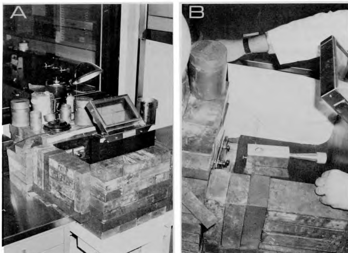
Fig. 6. Radium storage and handling facilities at Hahnemann Medical College and Hospital. A. General area is well lighted, with a ventilating hood on the right. B. Use of special brachytherapy tools. Shown is use of a special vise to hold a radium source vertical during string attachment. A special threader used to insert the string and long forceps help assure hands are several inches from the source at all times.
