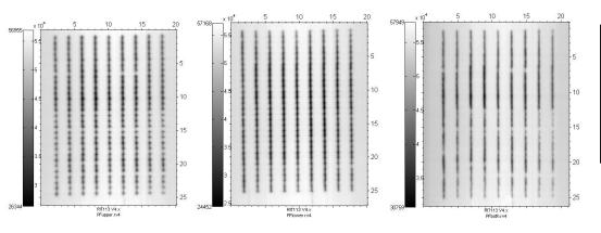
The double-stack MLC system has adequate RF shielding, an overall less inter- and intra- leaf transmission, and a good agreement with TPS on output factor prediction. Picket fence is a good test to evaluate the positioning accuracy for both layers individually.
