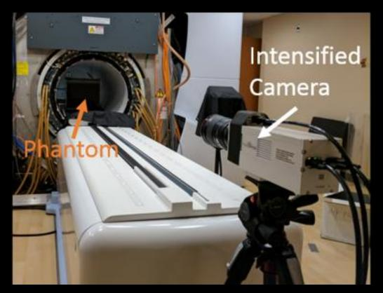
In this work, ERE was measured for the first time on an MR-linac using a novel optical method (scintillation and Cherenkov excited fluorescence) in phantoms. This method allows for real-time, 2-D measurement of dose distributions without the need to perturb the beam and solid-air interface with a detector. Results suggest that it is possible that the TPS is under-reporting the extent of dose escalation due to ERE, as well as the localization of the dose escalation.
