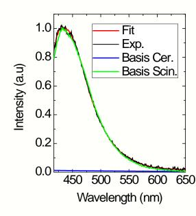
Čerenkov radiation is minimized in hollow core waveguides.
