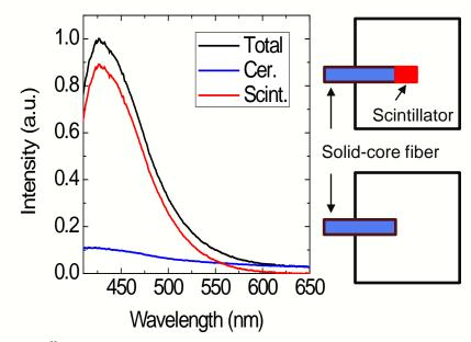
Čerenkov radiation contamination is a significant issue in fiber optic dosimetry using solid core fibers.
