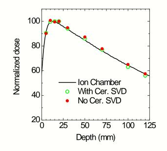
PDD measured by using the HWG with and without correction for Čerenkov radiation shows similar result.
